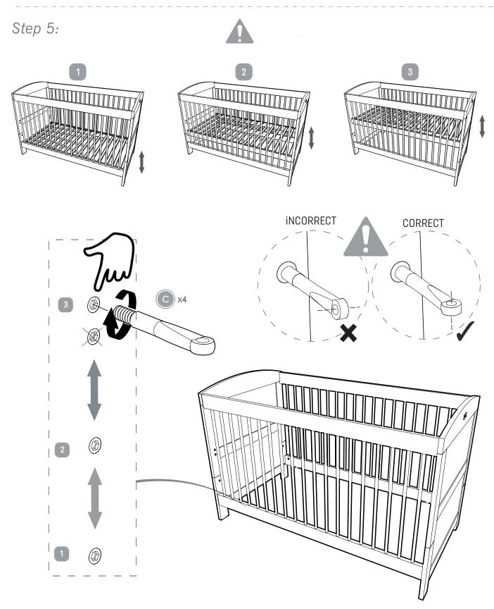
The cot bed base can be fitted at three different heights.
